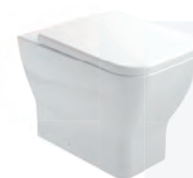
27110 BTW WC PAN FOR HIGH-LEVEL CISTERN 54 X 36 cm With dual outlet and fixing kit. Conversion bend needed for S-trap installation. Conversion bend not needed for P-trap installation.
